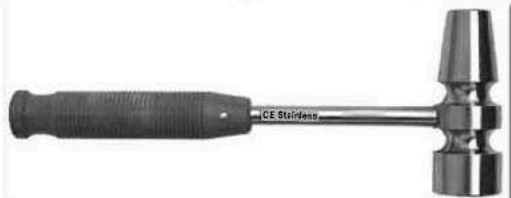
30-537-28 He-Man Mallet 28cm / 11" Head Dia 38mm / 24mm Weight 2lb (906gm)
